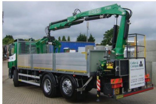
Left: one of Fassi's rear-mounted loaders on a flatbed truck with tag axle
