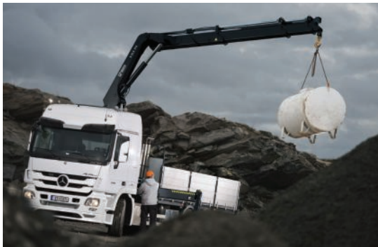
Right: Cargotec remote-operated truck crane Centre: stabiliser extensions ensure safe lifting
